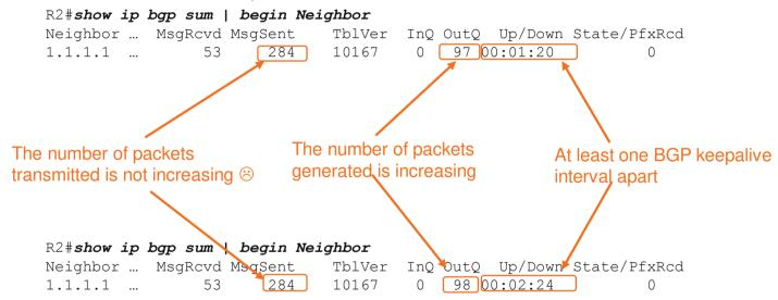
OutQ is incrementing due to keepalive generation MsgSent is not incrementing Something is "stuck" on the OutQ The keepalives are not leaving R2!!
